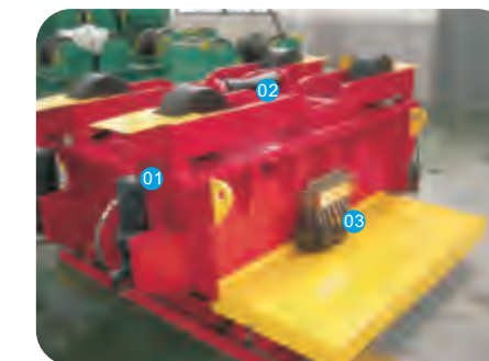
01 4只径向油缸 4 sets radial cylinder
