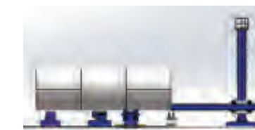
G、内外环缝焊接, 依次接长 G、 Inner & outer circular seam welding, jointing
