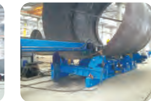
组对完成后由操作机焊接内外环缝 Welding inner & outer circular seam after finish fit up together
