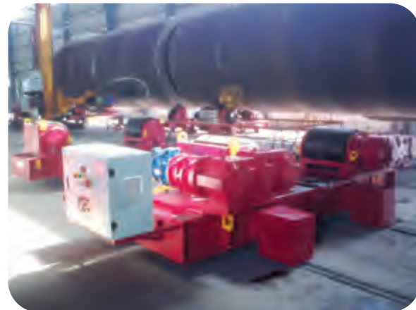
150T电动行走滚轮架 150T Motorized travel welding rotator
