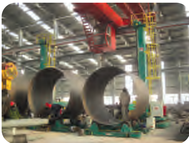
B、焊接内纵缝 B、Inner longitudinal seam welding
