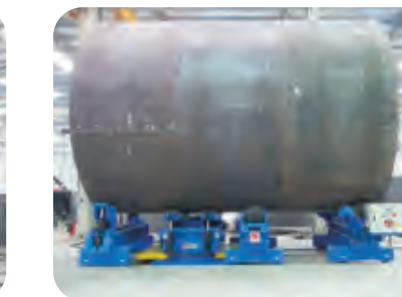
组对完成后由操作机焊接内外环缝 Welding inner & outer circular seam after finish fit up together
