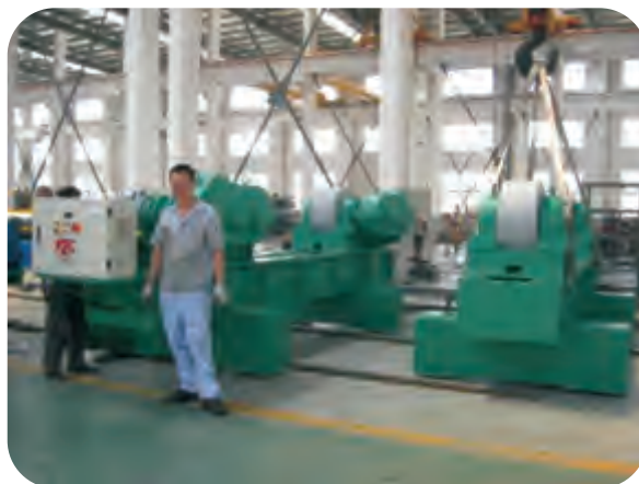
300T电动行走滚轮架 300T Motorized travel welding rotator
