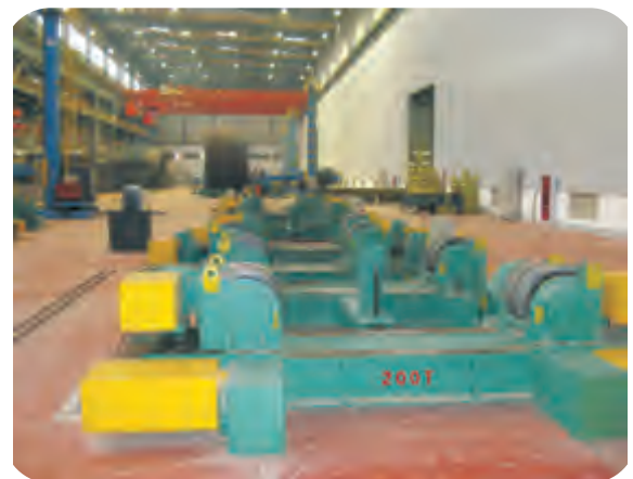
200T电动行走滚轮架 200T Motorized travel welding rotator
