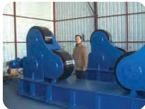
500T自调式滚轮架 500T Self-alignment welding rotator
